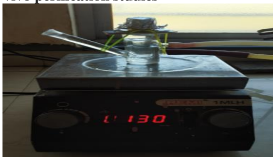
Figure 3: Ex-vivo permeation studies using human cadaver skin (Franz diffusion cell apparatus)
