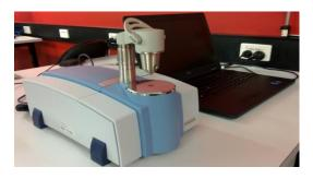
Figure 4: FT-IR Spectroscopy
