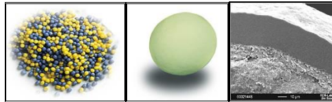
Figure 2: (a) Pellets, (b) Perfect pellet, (c) Coated pellet
