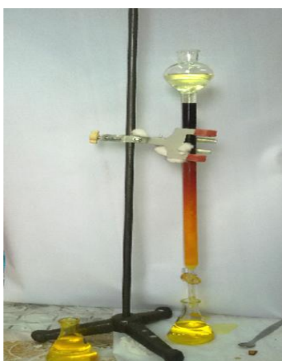
Figure 1: (a) Characterization of extract CUR through TLC- iodine plate, (b) & (c): Isolation of CUR through column chromatography
