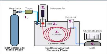
Gas chromatography (GC) begins vaporizing the sample, which is then injected into a chromatographic column. In this column, the sample moves alongside an inert gas, typically helium or nitrogen. As the sample travels through the column, its various components separate based interactions with the stationary phase inside the column. This separation occurs because different components have different affinities for the stationary phase, leading them to elute from the column at different times.
