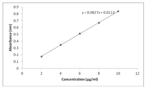
Fig. 4: Calibration curve of Metformin
